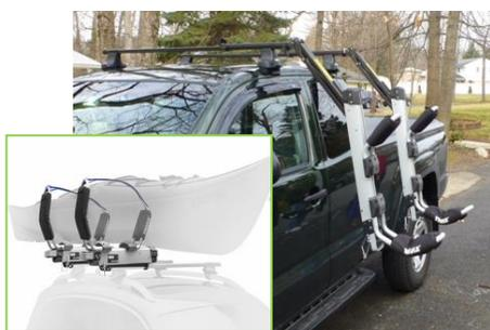
The most expensive method, but the easiest for one person, is the load-assist saddle system. These rack systems attach to the vehicle or rack system cross bars. They unlatch and swing down from the side of the vehicle so that the cradles are about waist high and vertically oriented. The kayak is simply placed onto the cradles on its side, strapped down, and then, with a spring assist, swung back onto the roof of the vehicle with the kayak ending up upright like a standard pair of saddles.
